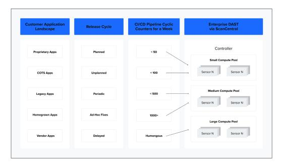
scanCentral DAST is a scalable architecture that enables Horizontally Scaling through multiple containerized versions of Weblnspect (known as Sensors) that can parallel process JavaScript, DOM Rendering, and other activities.
